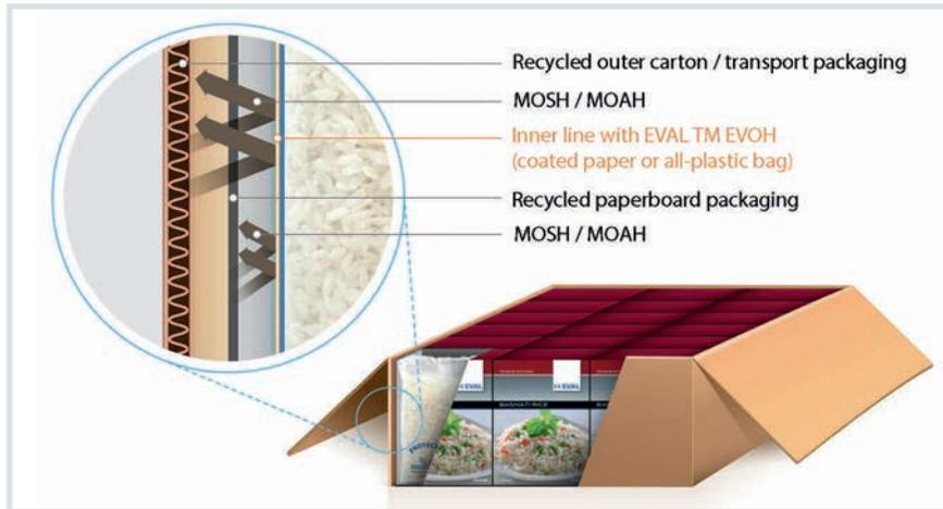
**Fig. 1.** A layer of only four micrometers of Eval barrier copolymer prevents impurities such as mineral oil from recycled cartons contaminating food (© Kuraray)
